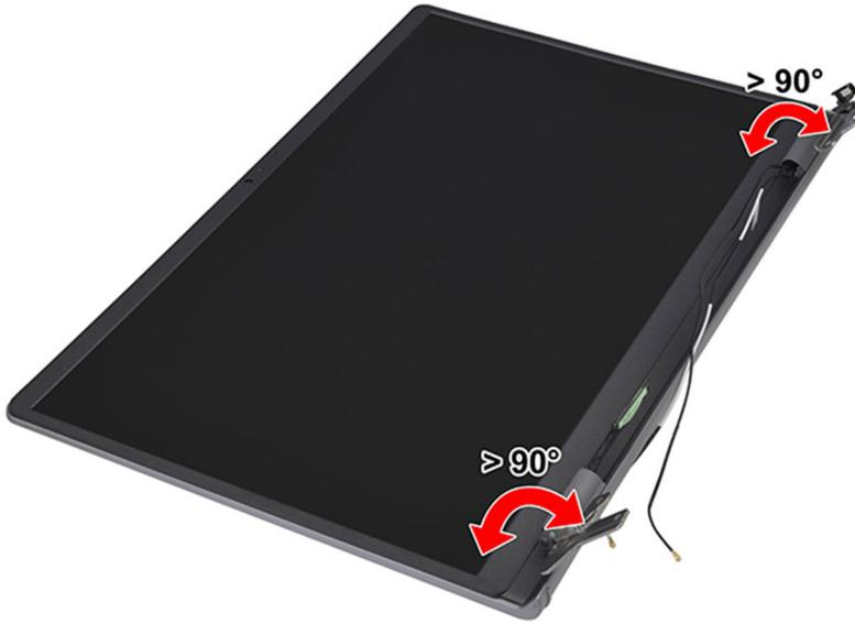
2. Using a plastic scribe, pry open the left display-hinge cap from its right side and remove it from the left display hinge.
