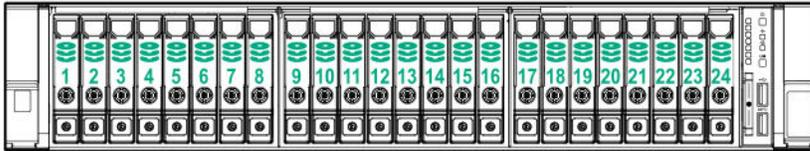
When any stacked 2SFF drive cage is connected to the SAS expander, the drive numbering skips the second number to allow **uFF drive bay numbering** on page 33. For example, when a rear 2SFF drive cage is connected to SAS expander port 9, then the drive numbers are 25 and 27.
