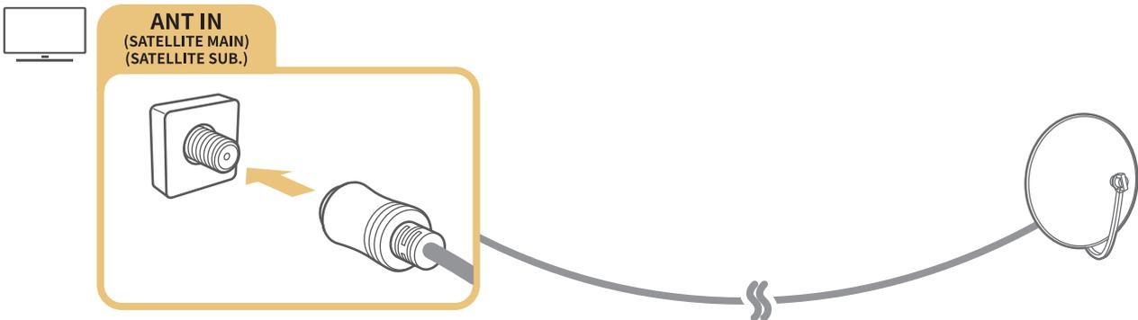
It is best to connect the both connectors using a Multi-Switch or DiSEqC. Switch, etc and to set **Aerial Connection Type** to **Dual Oscillator**.
